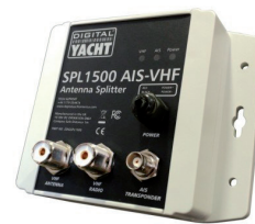
Use the SPL1500 - VHF Antenna splitter to share the vessels VHF Antenna with VHF and AIS.
